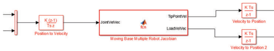
Figure 4: Simulink block diagram of the robot Jacobian
